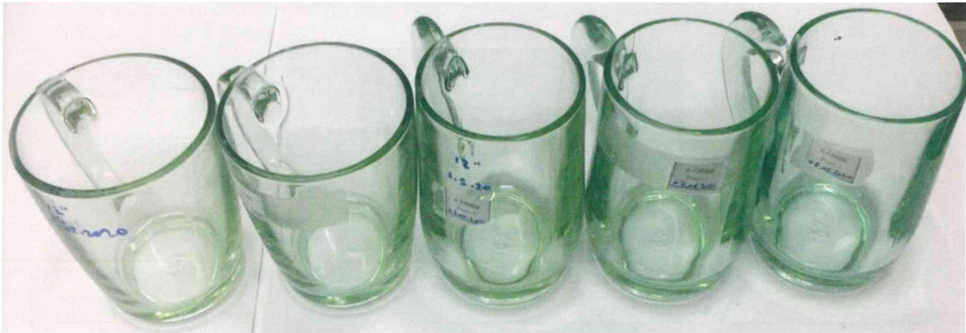
▲ Fig1. Standard soda lime and recycled glass products (increase in cullet ratio from 25→>95%).
