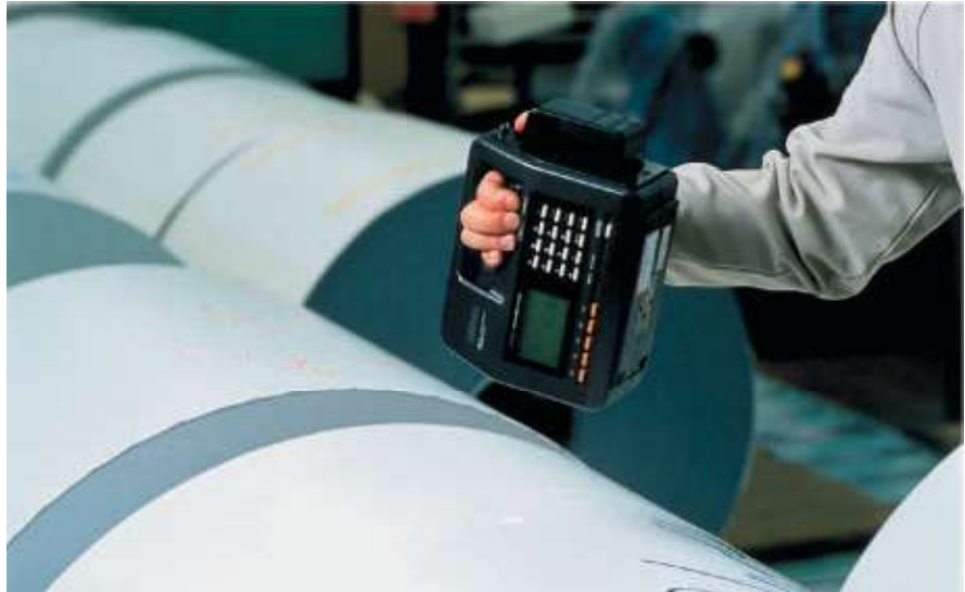
With Kett's KJT130 Handheld Portable Instant Moisture Meter, the user points the instrument at the product and the moisture content is instantly shown on a digital display.
