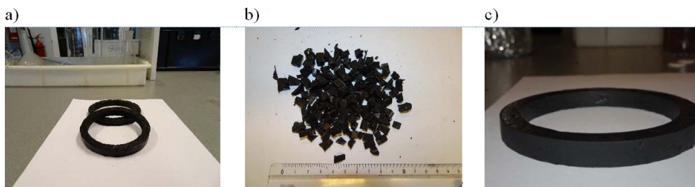
FIG. 2. — Recycling of DA crosslinked EPM-based O-rings: (a) freshly prepared rings; (b) ring after cutting up; (c) ring after recycling.
