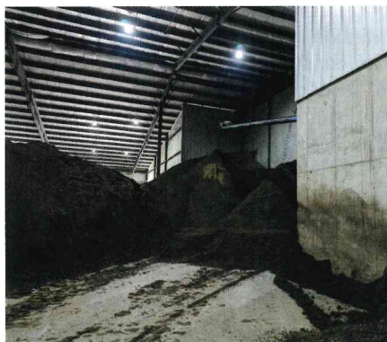
3. The leftover result of anaerobic digestion is a digestate that can be used for animal bedding and fertilizer. At the Middleton Digester, the digestate is dried completely before being returned for other uses at local farms. Courtesy: EnTech Solutions
