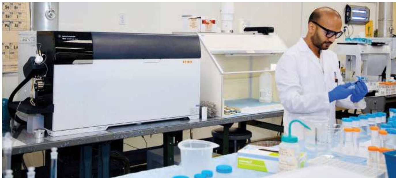
NJ Lab's Inductive Coupled Plasma Mass Spectroscopy is an instrument capable of detecting levels at parts per trillion (ppt) levels. Analyses performed by this device are preferred to satisfy USP testing requirements.
