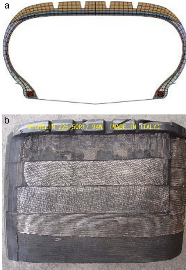
FIG. 8. — Structure of tire: (a) structure and material; (b) symmetrical tire steel belt.
