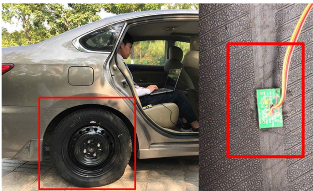
FIG. 1. — Intelligent tire system and data transmitted wirelessly.
