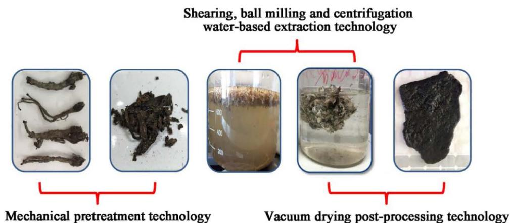
FIG. 6. — Water-based overall process.
