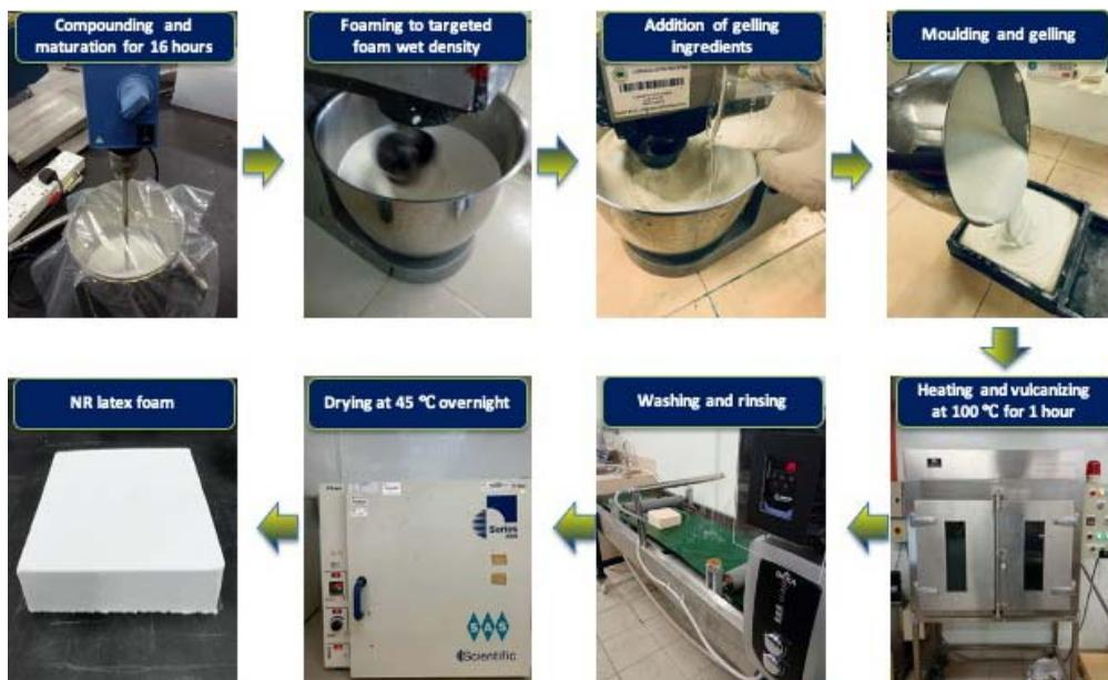
FIG. 2. — The different stages involved in the fabrication of NR latex foam using the Dunlop batch foaming process.
