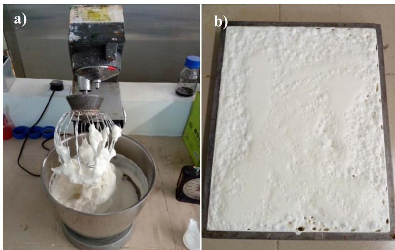
FIG. 5. — Failure during foaming process. (a) Foam coagulate; (b) Foam collapse.
