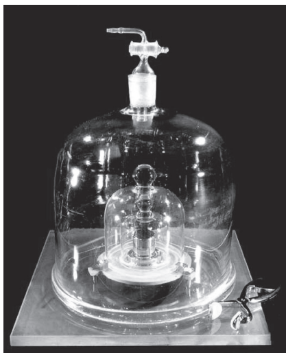
Figure 1 The international prototype of the kilogram at the International Bureau of Weights and Measures (BIPM). (2)
