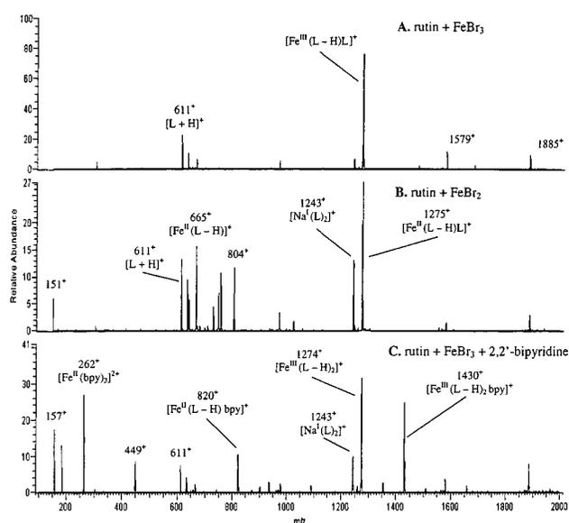
Figure 11. Comparison of rutin–metal complex formation with doubly and triply charged metal salts. The vertical scales are directly comparable for this series of spectra, with maximum abundance being 100, and values less than 100 signifying proportionally lower abundances.
