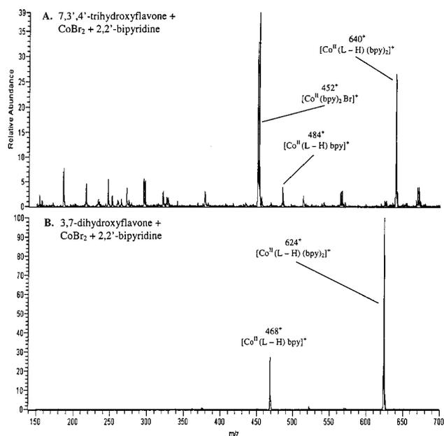
Figure 10. Comparison of ESI-MS of flavonoid model compounds with differing structural features that favor or discourage metal coordination. The vertical scales are directly comparable for this series of spectra, with maximum abundance being 100, and values less than 100 signifying proportionally lower abundances.
