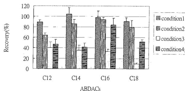
Figure 2. Extraction recoveries of ABDACs in various conditions as described in text. Extractions were performed on three replicates; standard deviation is reported as an error bar.
