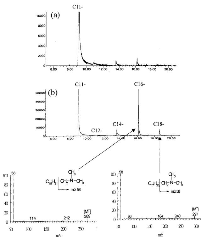
Figure 3. Extracted ion chromatograms (*m/z* 58) of ABDACs as their corresponding alkyldimethylamines and the internal standard (undecyldimethylamine) (a) prior to debenzylation and (b) after Hofmann degradation with potassium *tert*-butoxide at 90 °C; and their corresponding electron impact ionization mass spectra detected in the water sample from Kao-Ping river.
