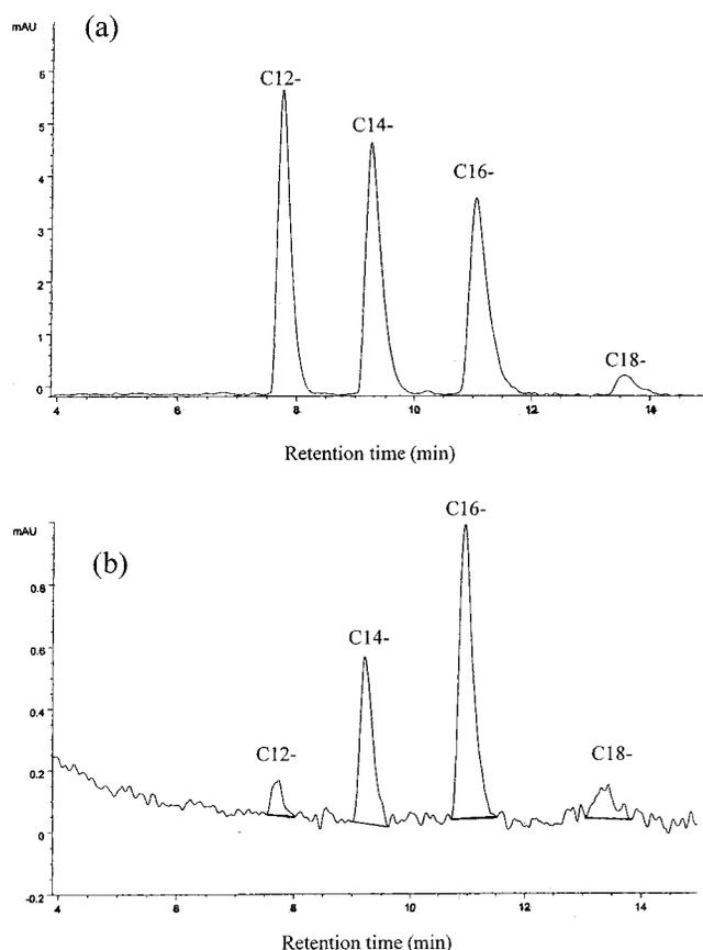
Figure 4. HPLC chromatograms for (a) standards containing C<sub>12</sub>–C<sub>18</sub>-ABDACs and (b) an RP-18 SPE extract of the water sample from Kao-Ping river. The corresponding concentrations are given in Table 2.
