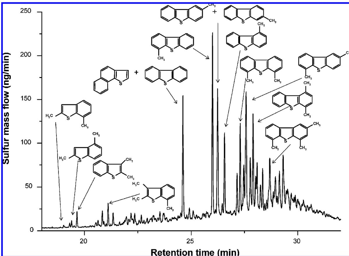
**Figure 2.** Sulfur mass flow chromatogram of vacuum gas oil sample BCR 107 with identified sulfur species by EI-MS.
