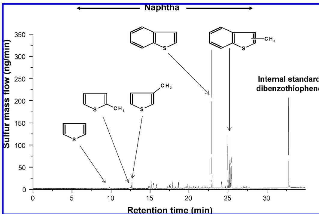
**Figure 5.** Sulfur mass flow chromatogram of the naphtha sample with identified sulfur species.
