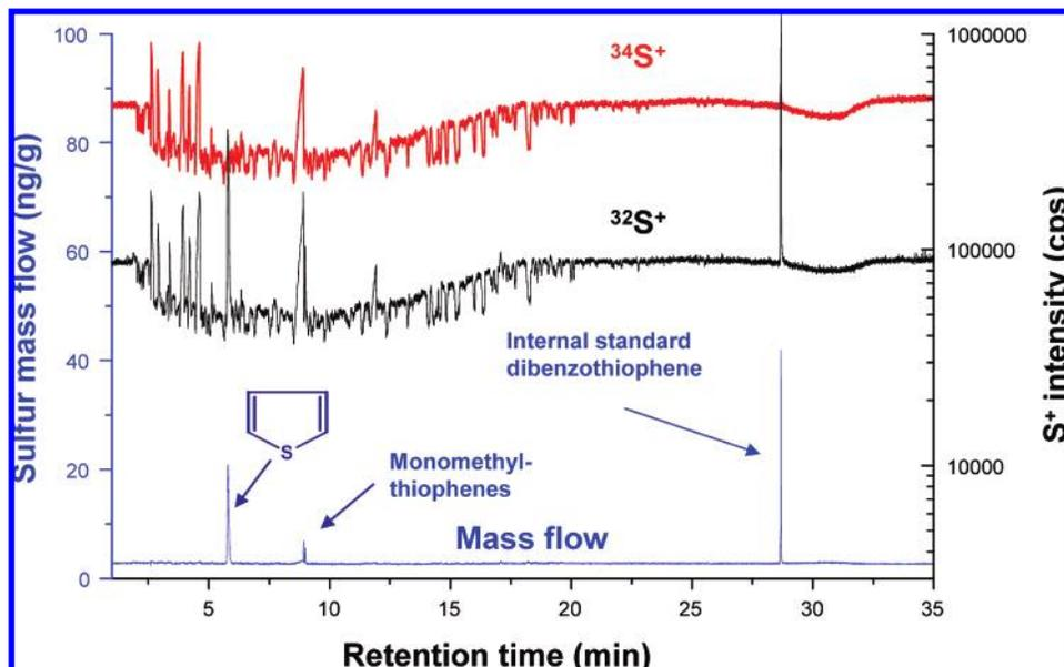
**Figure 4.** Measured sulfur ion intensity chromatogram (split ratio 3:1) of “sulfur-free” gasoline ERM-EF 213 demonstrating the influence of the hydrocarbon matrix at retention time interval of 2–21 min and representation of the matrix-independent sulfur mass flow chromatogram by GC–ICP–IDMS.
