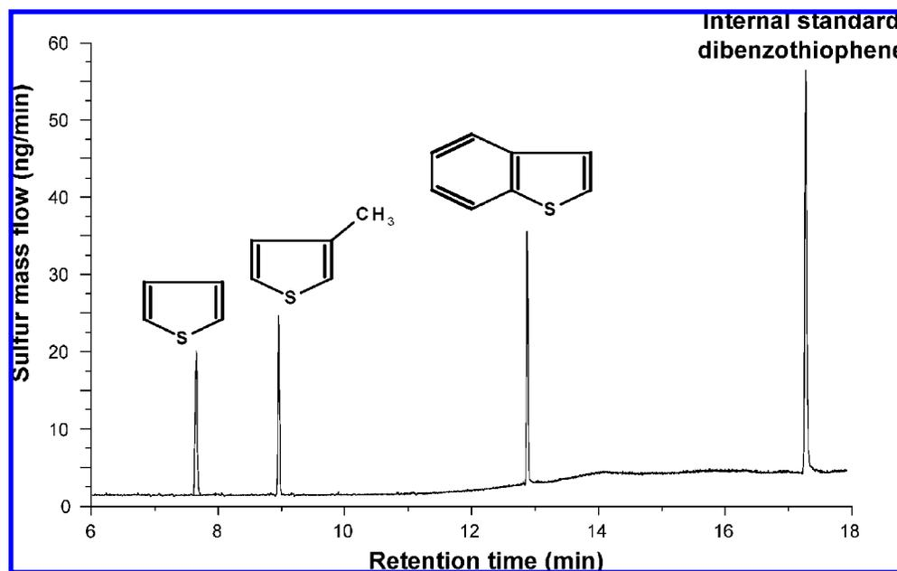
**Figure 3.** Sulfur mass flow chromatogram of standard reference material SRM-2296 containing three certified sulfur species.
