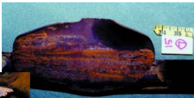
Above: Tube failure due to local overheating.
