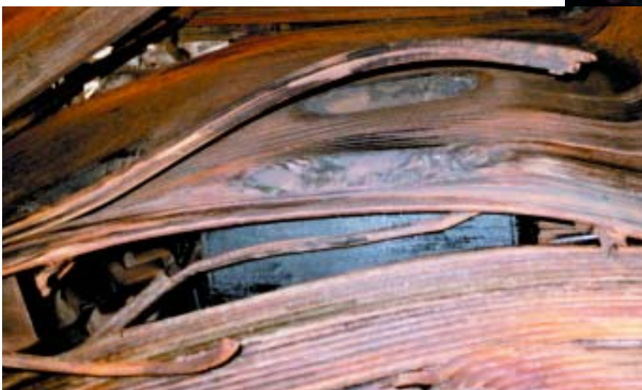
Above: Tube failure due to local overheating.
