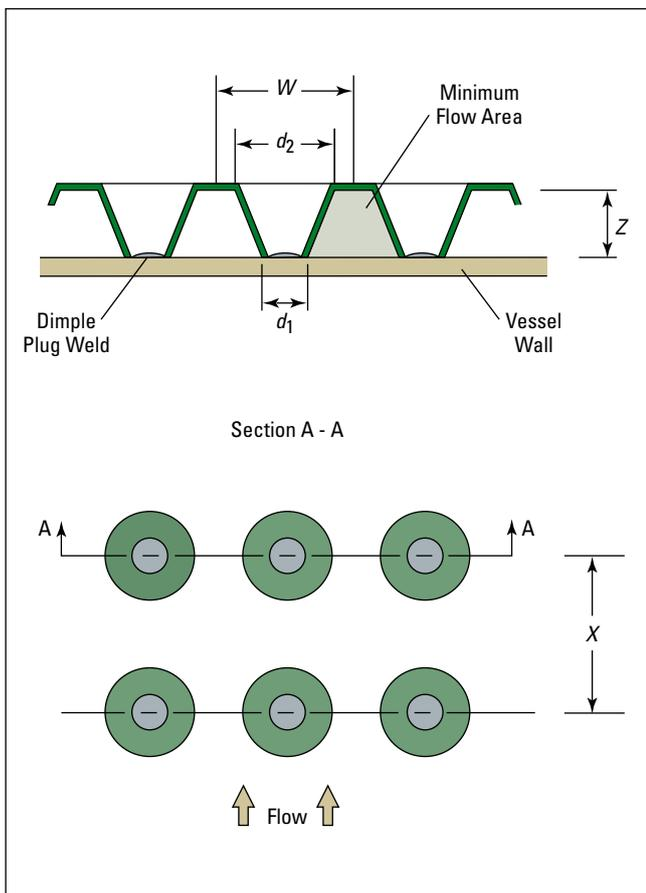
Figure 1. Dimple jacket geometry.
