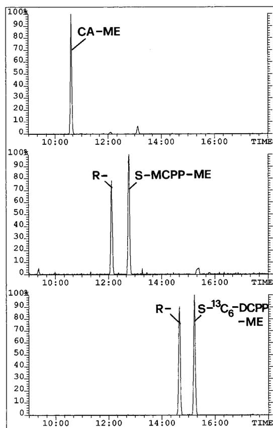
FIGURE 4. SRM chromatograms confirming the presence of CA ( $228^+ \rightarrow 128^+$ ; upper panel), and (*R*- and (*S*)-MCPP ( $228^+ \rightarrow 142^+$ ; middle panel) in the North Sea sample (sampling station S30, September 1996). Also shown, SRM chromatogram  $254^+ \rightarrow 168^+$  for  $^{13}C_6$ -DCPP (internal standard, lower panel). All compounds were analyzed as the methyl esters using the enantioselective OV1701-TBDM HRGC column.
