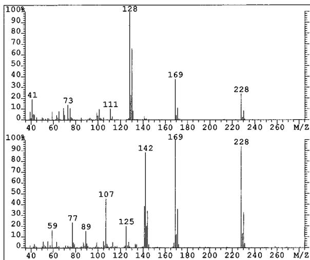
FIGURE 2. EI mass spectra of CA-ME (upper panel) and MCPP-ME (*R* enantiomer; lower panel). Note presence of isobaric  $\text{M}^+$  and  $(\text{M} - 59)^+$  ions and the diagnostically important “chlorophenol” ions at  $m/z$  128 and 142 for CA-ME and MCPP-ME, respectively.
