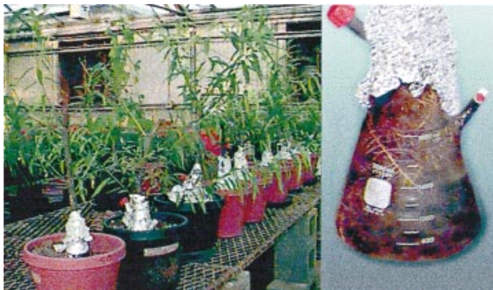
FIGURE 1. Photo of 6-month-old control and dosed rooted willow cuttings. The photo on the right shows the roots of willows in a dosed hydroponic bioreactor. The left port near the top of the reactor is for feeding and water replenishing, and on the right is the mininert sampling valve (modified from Burken and Schnoor (17)).
