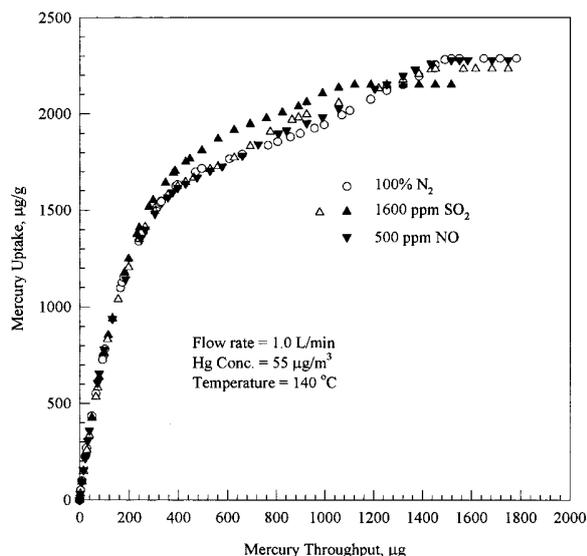
FIGURE 6. Effect of SO<sub>2</sub> and NO on mercury uptake by SIAC.
