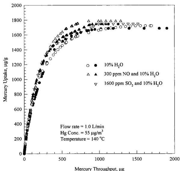
FIGURE 7. Effect of SO<sub>2</sub>/H<sub>2</sub>O and NO/H<sub>2</sub>O on mercury uptake by SIAC.
