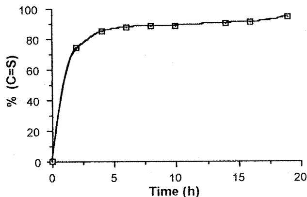
FIG. 4. Progress of the thionation reaction on crambe oil with LR/(C=O) = 0.5. See Figure 1 for abbreviation.
