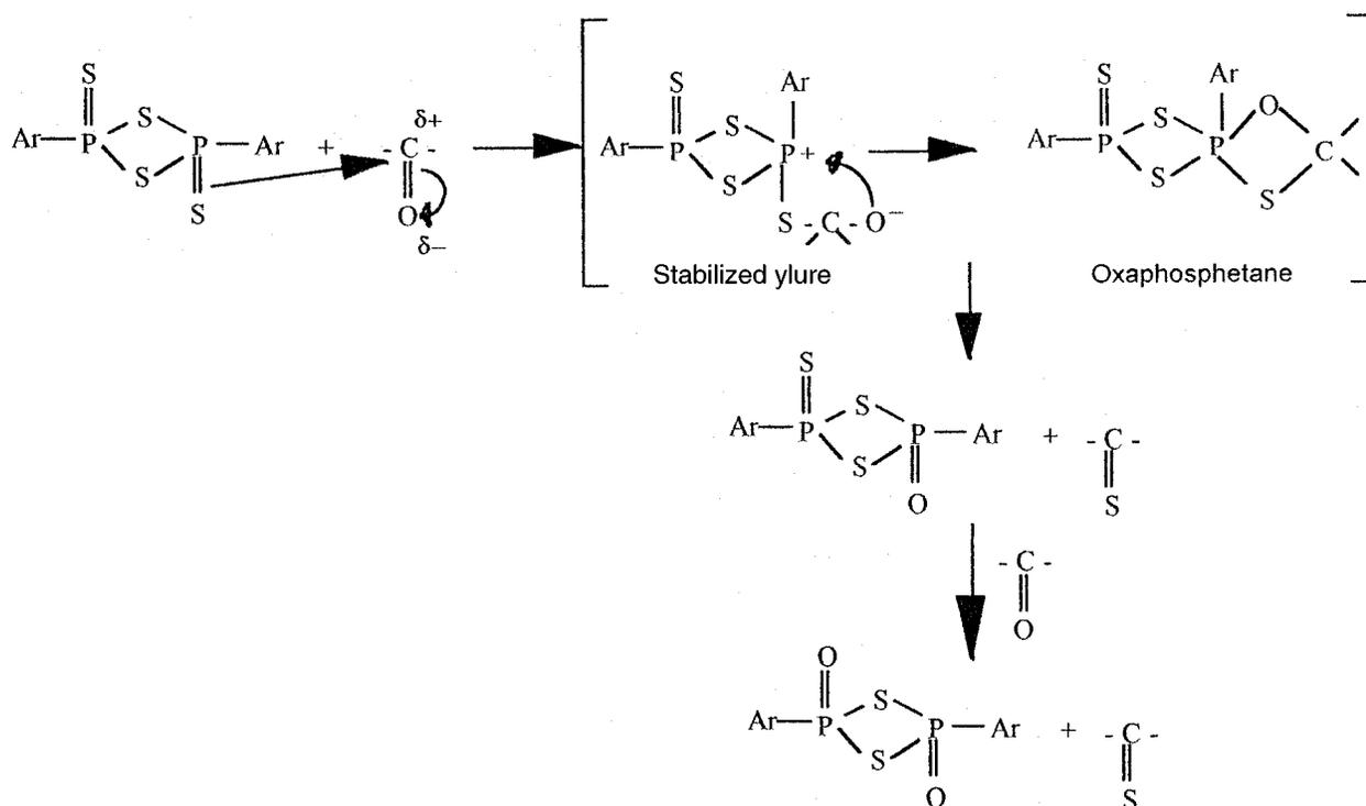
FIG. 5. Mechanism of thionation as a typical Wittig reaction.
