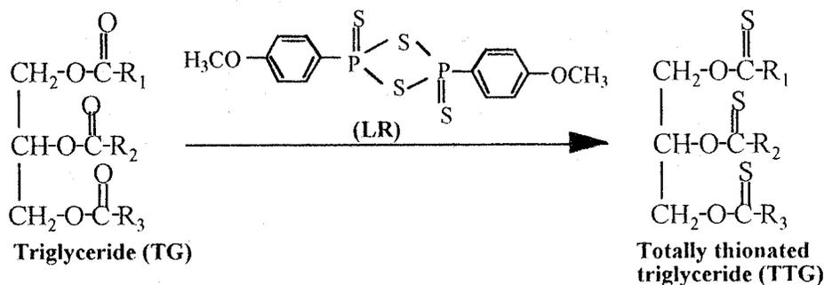
FIG. 2. Total thionation of a triglyceride (TG) (vegetable oil) using LR. See Figure 1 for other abbreviation.
