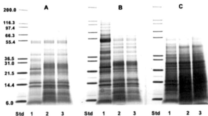
**FIG. 2.** Sodium dodecyl sulfate-polyacrylamide gel electrophoresis profiles of protein in supernatant fractions of DF (A), FFS (B), and FFU (C) bran samples. Std = molecular weight markers (kDa); lane 1 = whole bran; lane 2 = colloid-milled; lane 3 = colloid-milled + homogenized. See Figure 1 for abbreviations.
