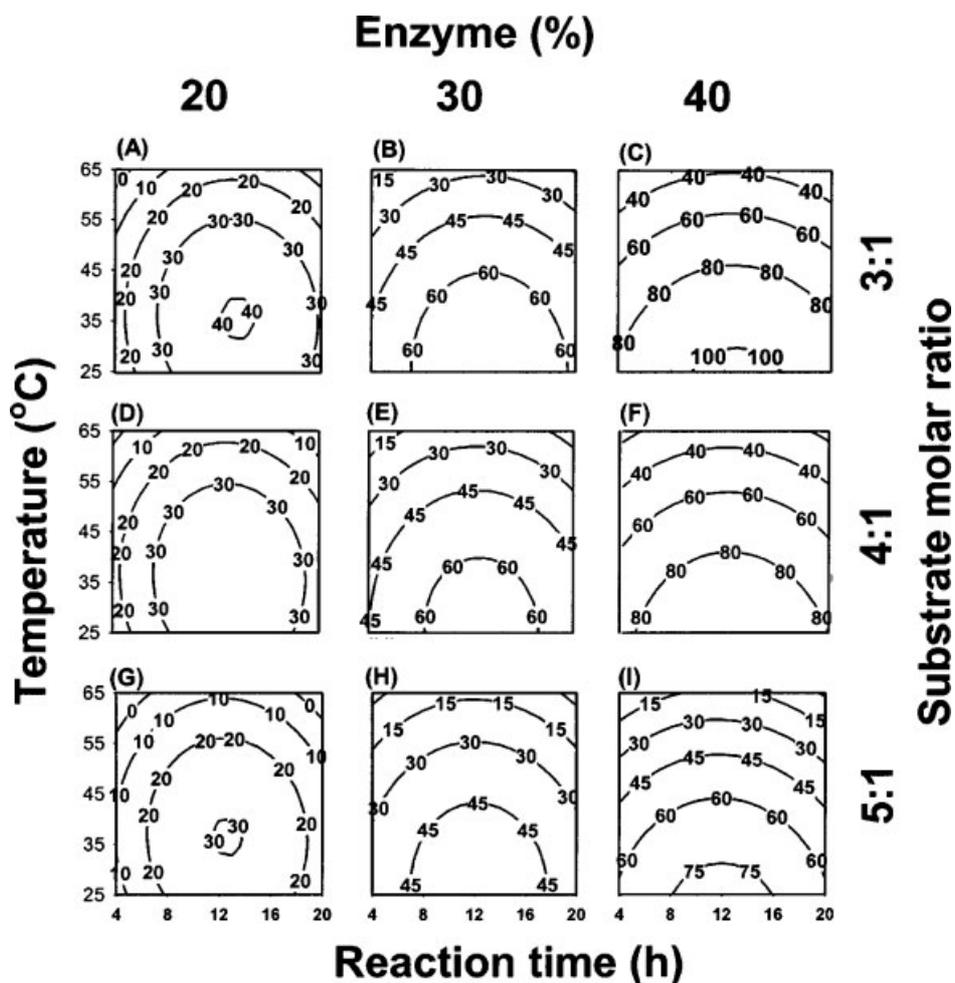
**Figure 4.** Contour plots of percent weight conversion of biodiesel. Enzyme concentration was by weight of canola oil and substrate molar ratio was methanol to canola oil. The numbers inside the contour plots indicate weight conversions at given reaction conditions.
