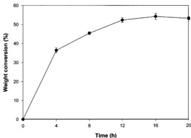
**Figure 1.** Time course of the alcoholysis of canola oil with methanol by Novozym 435. The reaction was carried out at 45 °C in 3 cm<sup>3</sup> hexane containing 1 g canola oil, substrate molar ratio of 4:1 (methanol:canola oil), 0.1 g (10%, w/w, weight of canola oil) Novozym 435. The activity of 10% Novozym 435 was 700 PLU.
