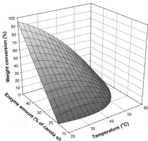
**Figure 2.** Response surface plot showing the effect of reaction temperature, Enzyme concentration, and their mutual interaction on biodiesel synthesis. Other synthesis parameters (reaction time, substrate molar ratio, and added water amount) are constant at 0 levels.
