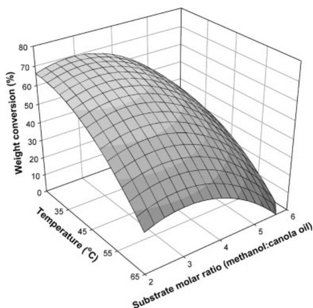
**Figure 3.** Response surface plot showing the effect of substrate molar ratio, reaction temperature, and their mutual interaction on biodiesel synthesis. Other synthesis parameters (reaction time, substrate molar ratio, and added water content) are constant at 0 levels.
