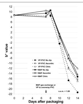
Figure  $5-b^*$  color of control, ascorbic acid-, or citric aciddipped pork chops with gas exchange modified atmosphere packaging or vacuum and overwrap packaging.
