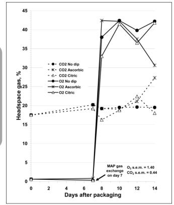
Figure 1—Headspace oxygen and carbon dioxide with gas exchange modified atmosphere packaging of control, citric acid-, or ascorbic acid-dipped pork chops.
