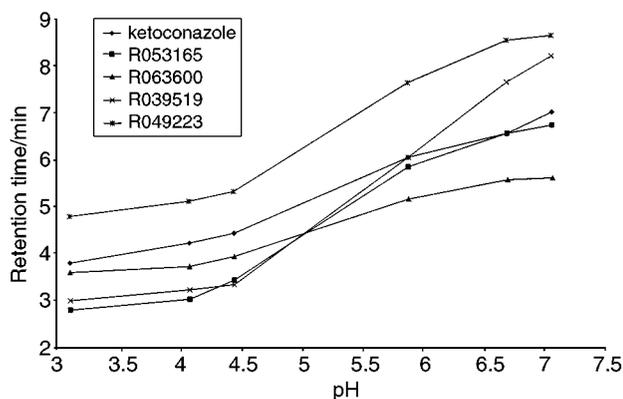
**Fig. 2** Variation of retention times of ketoconazole and impurities with pH of mobile phase. Mobile phase consists of 60% acetonitrile in 20 mM disodium hydrogen orthophosphate containing 0.2% diethylamine.
