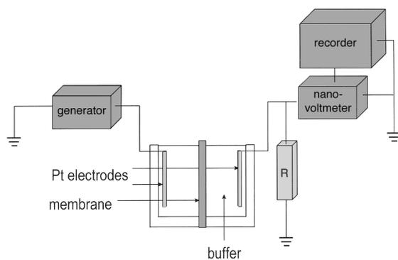
**Fig. 1** Schematic diagram of the experimental set-up for conductimetric measurements.
