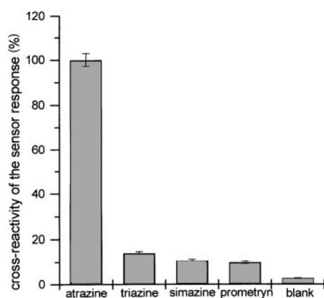
Fig. 6 Selectivity of the designed atrazine sensor. Atrazine-specific MIP membranes were influenced by atrazine, simazine, triazine and prometryn at a concentration of 70 nmol dm<sup>-3</sup>. Blank, response to 70 nmol dm<sup>-3</sup> atrazine of a sensor with the reference membrane. The measurements were carried out in 25 mmol dm<sup>-3</sup> potassium phosphate buffer (pH 7.5) containing 35 mmol dm<sup>-3</sup> NaCl. Each value represents the average of three independent measurements.
