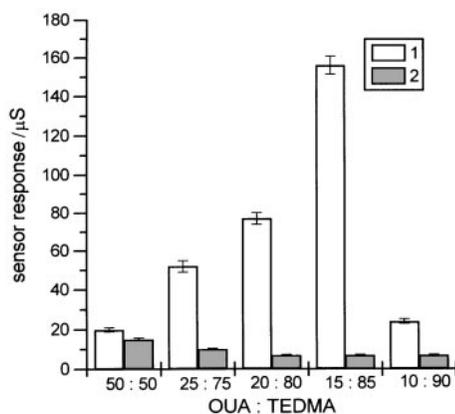
**Fig. 3** Responses to atrazine as a function of the cross-linking agent (TEDMA) concentration: (1) MIP membrane; (2) reference membrane. The measurements were carried out in 25 mmol dm<sup>-3</sup> potassium phosphate buffer (pH 7.5) containing 35 mmol dm<sup>-3</sup> NaCl. The responses were initiated by adding 60 nmol dm<sup>-3</sup> atrazine. Chloroform was used as a porogen. Each value represents the average of three independent measurements.
