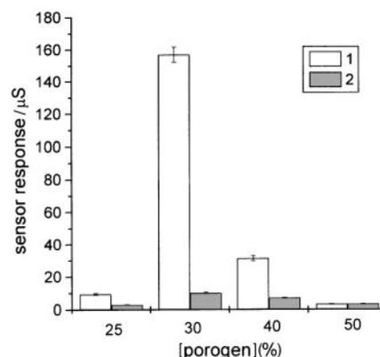
**Fig. 4** Responses to atrazine as a function of the porogen concentration: (1) MIP membrane; (2) reference membrane. Chloroform was used as a porogen. The measurements were carried out in 25 mmol dm<sup>-3</sup> potassium phosphate buffer (pH 7.5) containing 35 mmol dm<sup>-3</sup> NaCl. The responses were initiated by adding 60 nmol dm<sup>-3</sup> atrazine. Each value represents the average of three independent measurements.
