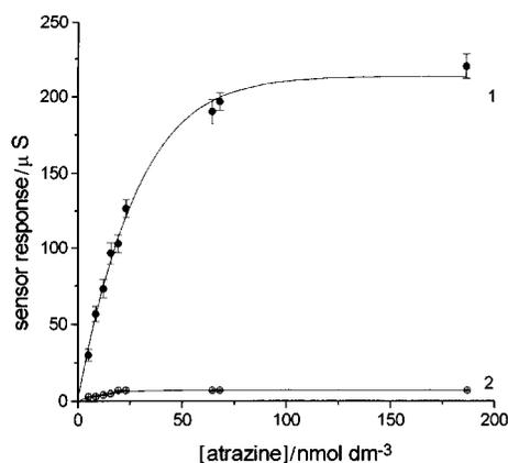
**Fig. 2** Magnitude of conductimetric responses caused by different concentrations of atrazine in (1) MIP membrane and (2) reference membrane. The measurements were carried out in 25 mmol dm<sup>-3</sup> potassium phosphate buffer (pH 7.5) containing 35 mmol dm<sup>-3</sup> NaCl. Each point represents the average of three independent measurements.
