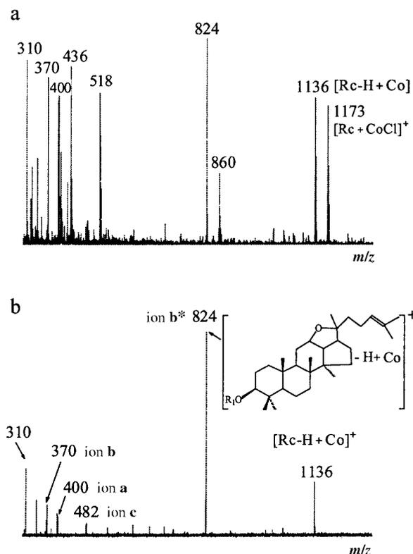
Fig. 3 Positive ion ES mass spectrum of ginsenoside Rc and  $Co^{2+}$  (a) and the CID mass spectrum of the  $[Rc - H^+ + Co^{2+}]^+$  ion at  $m/z$  1136 (b).
