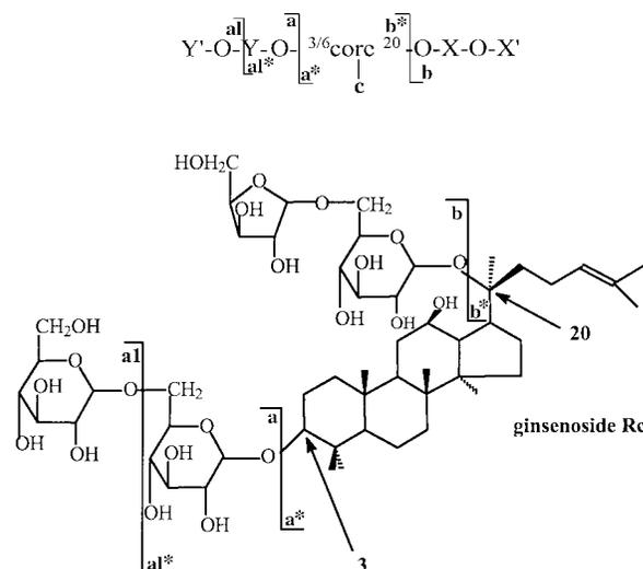
**Scheme 2** Main fragmentation pathways in the CID mass spectra of ginsenoside metal-attachment ions (see text and Table 1).
