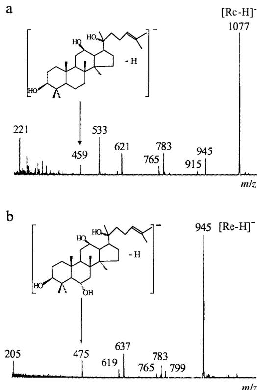
**Fig. 1** Negative ion ES mass spectra of ginsenoside Rc (a), and ginsenoside Re (b).
