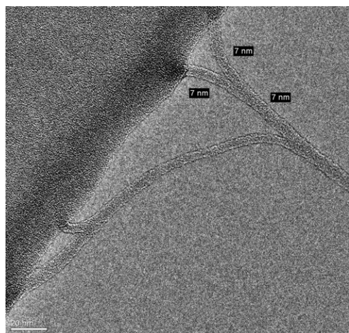
Fig. 9 TEM image of SWCNTs after coating with NOSC polymer. Bar represents 20 nm.
