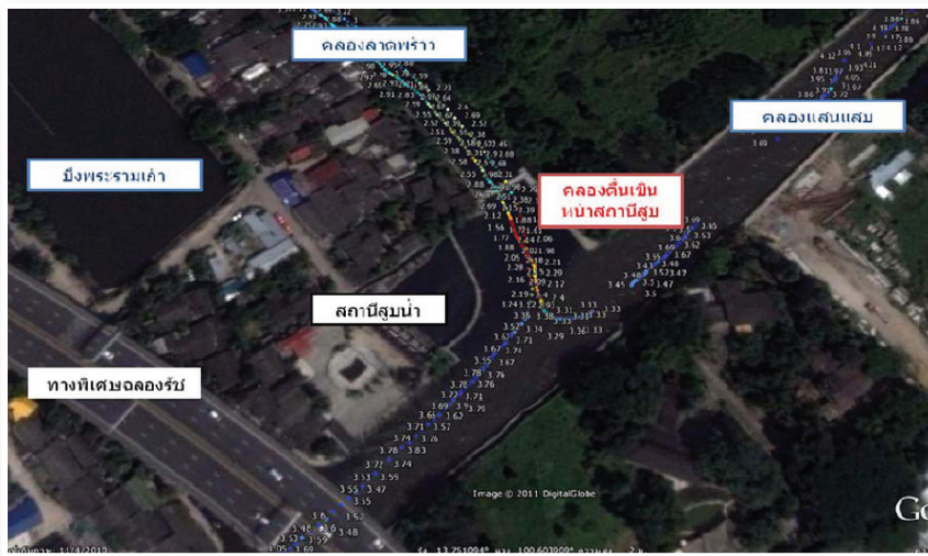
Figure 14 Example of the information giving out to the Army's Armed Forces Development Command. It is composed of GPS points and the depth information at each point plotted on Google Earth. As shown in the figure, the area near the junction point of Klong Ladprao and Klong Sanseab has shallow patch which needs to be cleared out for better drainage.
