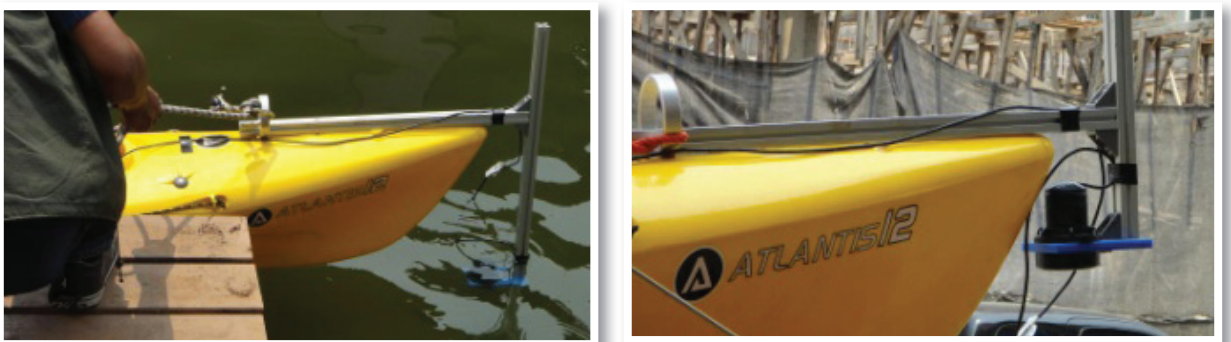
Figure 11 Echo sounder head and its installation at the bow of the kayak boat. The left figure shows the head during the deployment. The right figure shows the head in stowing position
