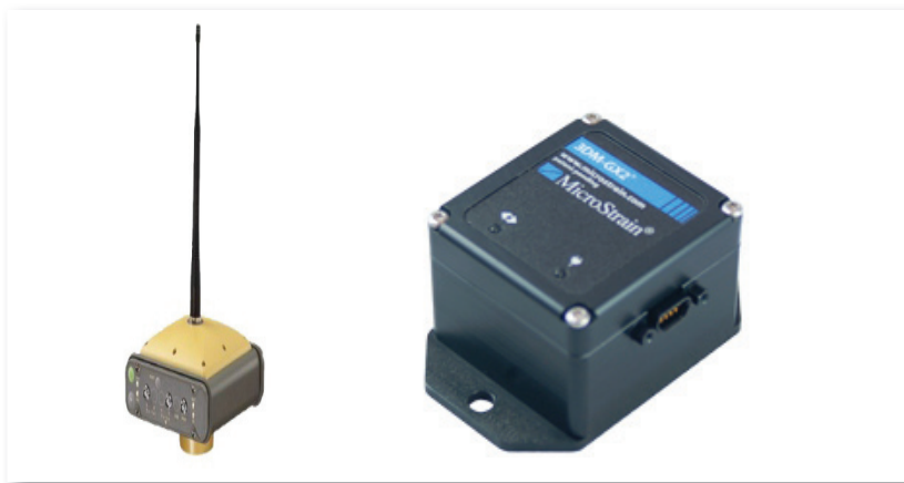
Figure 7 Two kinds of navigational sensors are used to control the robot in auto mode. RTK-GPS receiver from TOPCON Model Hiper GA (left) and IMU from MicroStrain Model 3DM-GX2 (right). A GPS gives real-time location of the robot boat. An IMU gives real-time heading angle information.
