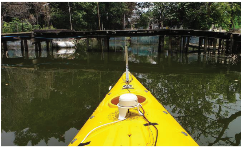
Figure1 Canals around Bangkok Metropolitan are shallow, narrow and usually are crossed by low clearance bridges. Therefore, small draft and low clearance are the two important specifications of the robot boat. Robot in the kayak form has no problem getting through this environment.
