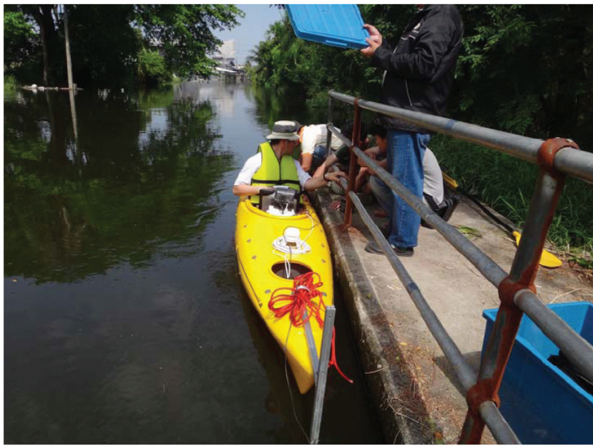
Figure 15 We used the kayak boat in manual mode equipped with echo sounding system to survey Bangkok Metropolitan's canals during the 2011 Thailand's great flooding. The system helped identifying the shallow spots. Such information was useful for pin pointing the digging operation in order to clear the canals for effective drainage of the flood water.
