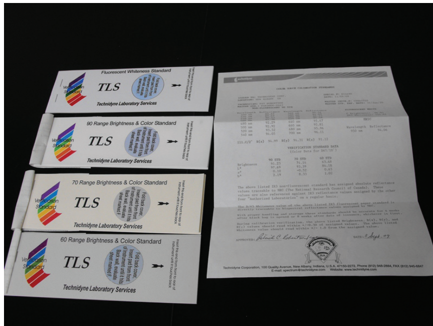
Figure 10 One set of Technidyne Laboratory Services' Paper Tabs (reference paper) consists of one pack of fluorescence paper, one pack of brightness 90 paper, one pack of brightness 70 paper and one pack of brightness 60 paper, and a certification states the issued values.
