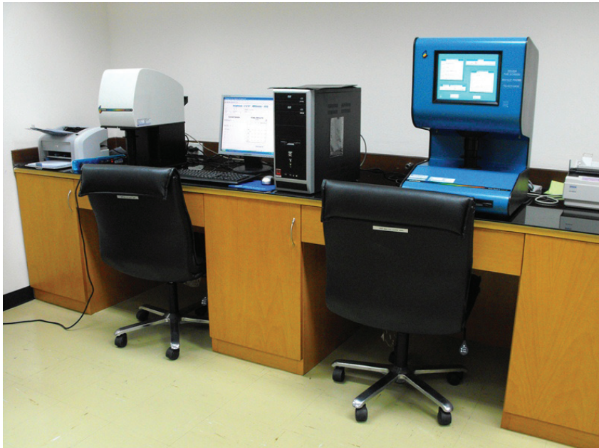
Figure 12 Brightness testers in Pulp and paper subdivision of the Physics and Engineering division of Department of Science Services' Optical laboratory; Colour Touch PC (left) and Colour Touch (right).
