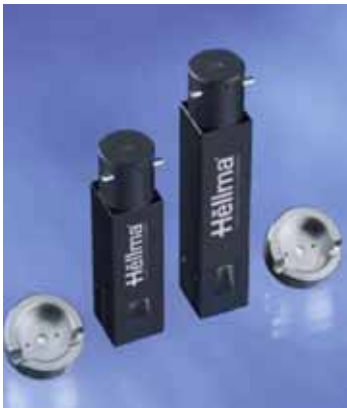
TrayCell Fiber optic ultra-micro measuring cell for sample volumes 0.7 – 5 \mu l (0.2 or 1 mm path length)
