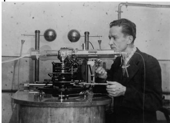
Figure 4.1.1.6 Professor Evgenii A. Porai-Koshits (1907-1999) with a wide-angle X-ray diffractometer used for phase analysis (photograph taken during the early 1950s).
