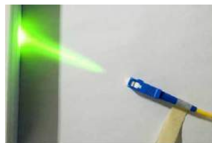
Green Fiber Laser (Toyota TI)
