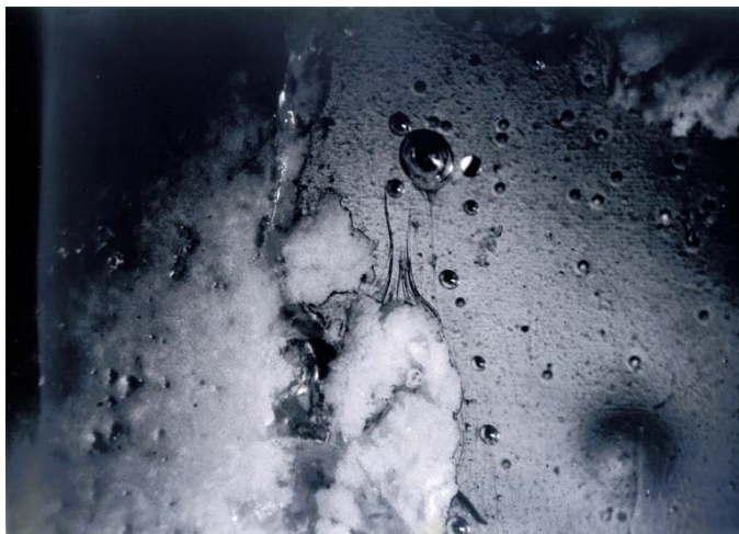
Fig. 4.2.4.1: Boundary layer area of a fused cast AZS 32 / soda lime silicate glass melt after a crucible test with generated glass defects, like Stones, Knots and Blisters.
