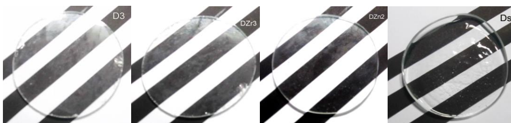
Fig 2. Image of glass specimens after weathering.
