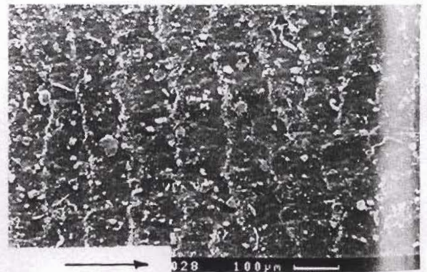
Fig. 8 SEM photograph of abraded surface of compound H1.
