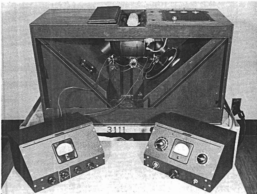
FIG. 5.—The experimental photoelectric photometer adapted to measure the excitation purity of the color of yellow sweet corn.
