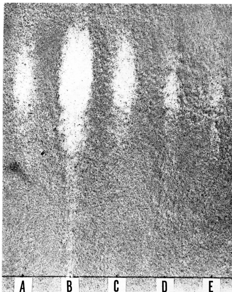
Fig. 7.—Paper chromatograms developed in system 2 showing the Phosdrin obtained from 2.5 g samples of lettuce at various times after spraying with Phosdrin. A, 5 \mu g Phosdrin. B, 4 hours. C, 1 day. D, 2 days. E, 3 days.
