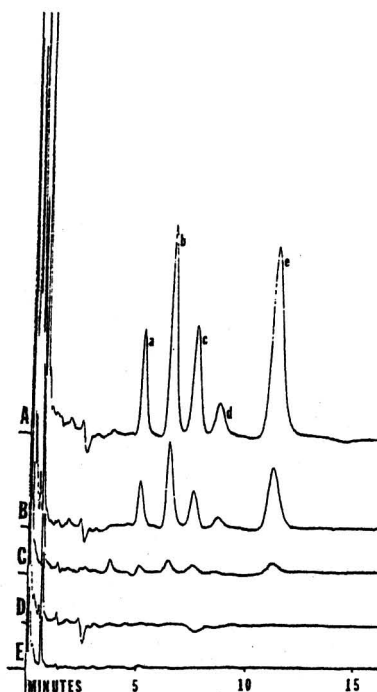
FIG. 2—Electron capture GLC chromatograms from eluate B. GLC conditions given under Apparatus ; injection equivalent to 57 mg sample for all chromatograms. A, 8 g corn oil fortified at following ppm: a. heptachlor epoxide 0.01, b. endosulfan I 0.02, c. dieldrin 0.013, d. endosulfan II 0.008, e. endosulfan sulfate 0.05; B, 8 g corn oil fortified at one-half levels in A; C, reagents (no oil) fortified equivalent to one-tenth levels of A; D, 8 g corn oil (not fortified); E, reagent blank.
