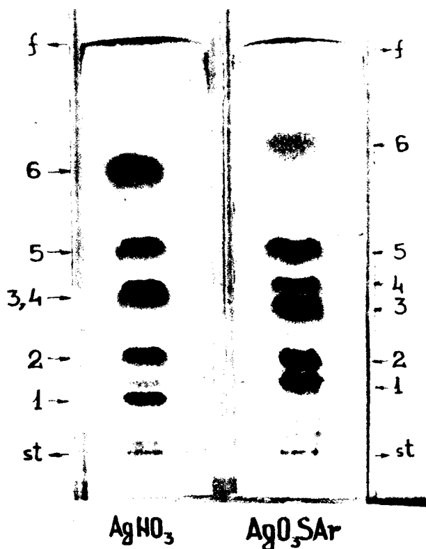
Fig. 1. Chromatography of the fatty acid methyl esters on silver nitrate and silver benzenesulfonate ( \text{AgO}_3\text{SAr} ) impregnated silica-gel layers:
