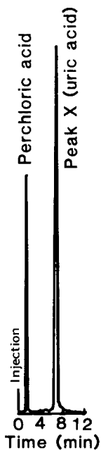
Figure 2. The typical reversed-phase high-performance liquid chromatogram, obtained by injecting 10 \mu\text{l} of the deproteinized human serum into the RPHPLC-ECD system. Ten microliters of the serum was injected into a column (Finepak SIL C18, JASCO) by using a microsyringe. The eluent was 0.2 M phosphate buffer ( \text{KH}_2\text{PO}_4\text{-H}_3\text{PO}_4 , pH 2.0). The column temperature was maintained at 35^\circ\text{C} . The flow rate was 0.5 ml/min. Eluate from RPHPLC was electrochemically monitored by aid of an electrochemical detector under the potentiostatic condition (+800 mV vs. \text{Ag}/\text{AgCl} ). The sensitivity of the detector was set at 64\text{ nA} full scale. For further explanations, see the text.
