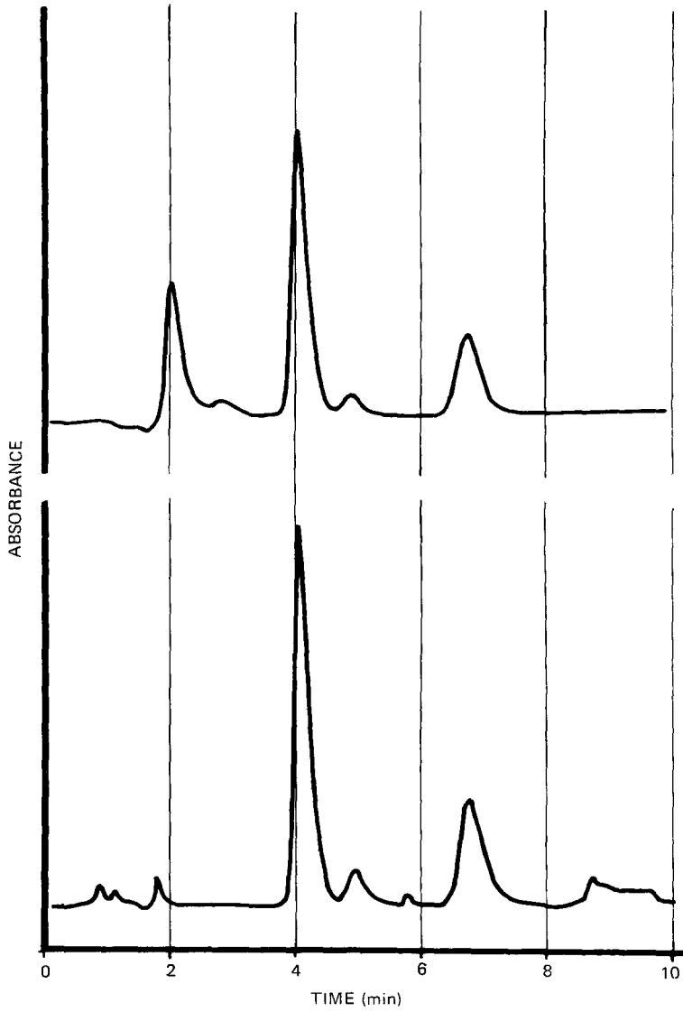
FIGURE 6. Comparison of LCO 2 and Commercial Pyrethrum Extracts. Upper - LCO 2 extract. Lower - Commercial extract. HPLC conditions - see Figure 5.
