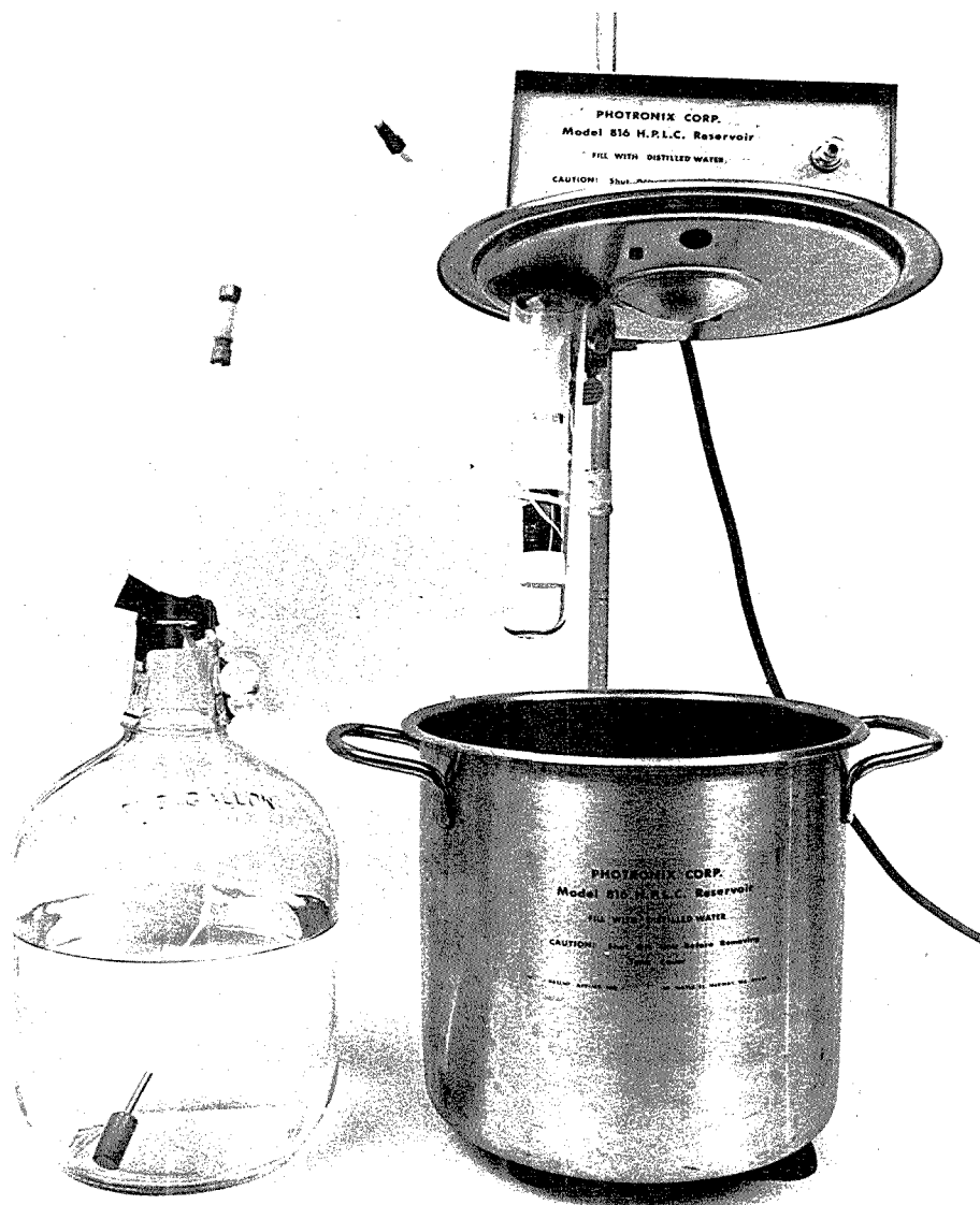
FIGURE 1. Photronix HPLC reservoir with the lid raised to show the Teflon tubing for the flow-through UV irradiator coiled around the lamp and running to an auxiliary flask of distilled water.
