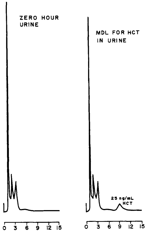
Figure 8. HPLC Chromatograms of extracts of a zero-hour equine urine (left) and a zero hour equine urine spiked with 25 ng/ml hydrochlorothiazide (right) This level of HCT in urine represents the practical minimum detectable limit.
