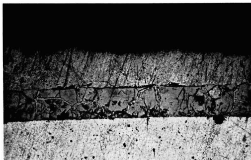
Fig. 13. Photomicrograph of a typical iron-molybdenum deposit. Magnification 500X before reduction for publication.
