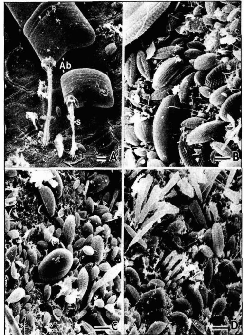
Figure 2—(A) Achnanthes brevipes (Ab), a tolerant diatom species. s, stalk; (B–D) Fouling after three months. (B) Control, aluminum vinyl (Al); (C) Tributyltinfluoride antifouling paint (TBTF); (D) Antifouling wax (AW). Bar, 10 \mu m
