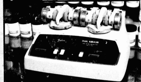
TOP: Reactor produces developmental polyethylene waxes. MIDDLE: Samples are prepared by roller, brush, draw-down and spray application techniques. BOTTOM: Testing is conducted for slip and friction, rub and mar, and wear and abrasion.*
