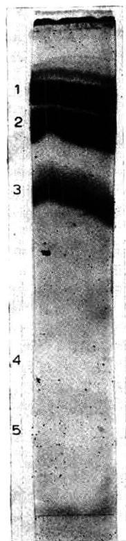
Fig. 2. Partition chromatogram of monoglycerides. For the conditions of separation and development see "EXPERIMENTAL: Chromatographic separation of monoglycerides". Sample weight 1000 \mu g. 1 = Monolinolenin; 2 = monolinolein; 3 = monoolein; 4 = monopalmitin; 5 = monostearin.
