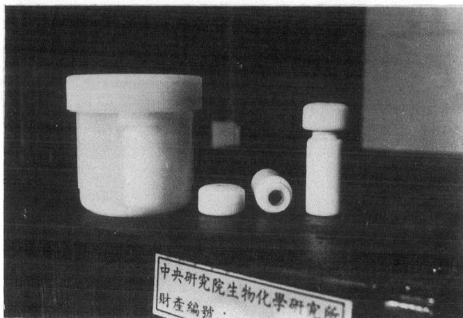
Fig. 1. PTFE vials and container shown inside a commercial microwave oven. The thicknesses of the two PTFE vials (right) and the container (left) are 6 and 5 mm, respectively. The container is 7.5 cm high with I.D. 7.5 cm and the vials are 5.5 cm high and with O.D. 3.0 and I.D. 1.8 cm. At the top of the small vial, a sealing septum of silicone-rubber was attached (not shown) for insertion of a needle to flush the vial with inert gas (e.g., nitrogen) before the microwave heating. The container can contain 1–5 vials at one time. It is preferably placed at the same location to ensure constant and reproducible heating.
