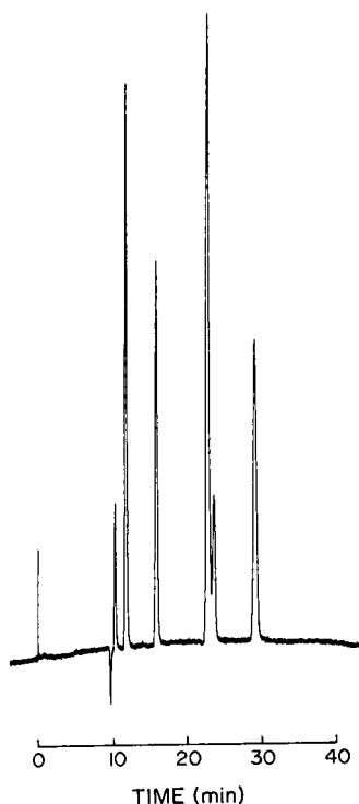
Fig. 1. Chromatogram illustrating refractive index artifact occurring in absorbance detection upon injection of standard test mixture dissolved in methanol into a methanol-water (75:25, v/v) mobile phase. Characteristic derivative-shaped response from absorbance anomaly is seen at a retention time of 10 min.
