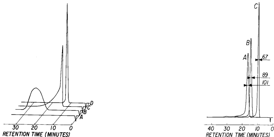
Fig. 2. Effect of different eluent compositions on chromatography of IDA: (A) 0.5 mM bicarbonate, pH 8.3; (B) 0.5 mM bicarbonate + 0.84 mM 4-cyanophenol, pH 8.3; (C) 0.2 mM carbonate + 0.84 mM 4-cyanophenol, pH 9.5; (D) 1.15 mM carbonate + 0.84 mM 4-cyanophenol, pH 10.2. A 20- \mu l volume of IDA standard solution (120 mg/l) was injected.
