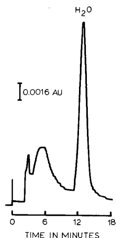
Fig. 3. Spectrum of 0.138% water in a methanolic solution of 1.15 M 3-mercaptopropionic acid. Sample loop, 20 \mu l; separation column, 10 cm \times 8 mm I.D.; flow-rate, 1 ml/min. Other conditions are given in the text.
