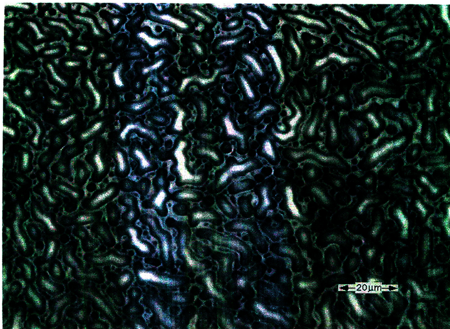
Fig. 6. Optical microscopy image of the deposit morphology of the polystyrene NBS 706 sample on the Ge-Al collection disk corresponding to Figs. 2, 7, and 8.
