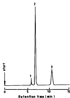
Fig. 3. Chromatogram of a typical mixture containing (1) DASA (2 \mu\text{g} ), (2) AASA (20 \mu\text{g} ) and (3) DABA (5 \mu\text{g} ).
