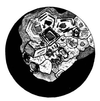
Fig. 10. Gold bearing garnet ore from Ta Tago, showing octagonal, hexagonal and square cross sections of garnets between crossed nicols.
