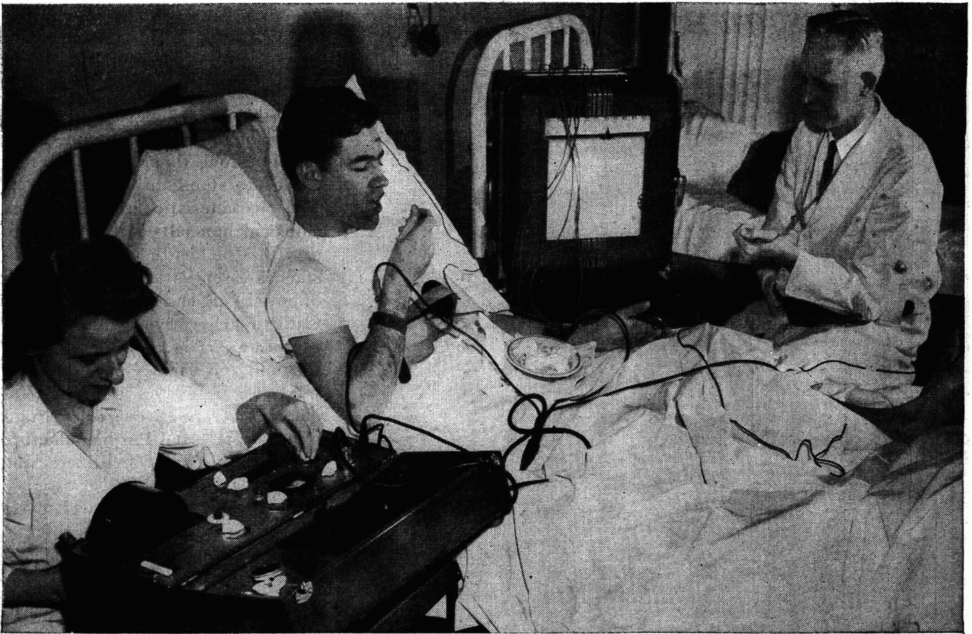
For testing the effect of food temperature on the flow of blood, Dr. Austin Henschel (right), Assoc. Prof. of Physiological Hygiene at Univ. of Minnesota, uses a Speedomax Recorder to check skin temperature of a student eating ice cream.
