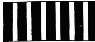
9812-V, Fig. 2. Showing Stroboscopic lines as seen through window openings when timer is in motion and adjusted to 200 r.p.m.
