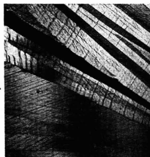
Figure 2. Fusion Preparation of Adipic Acid Crossed Nicols
