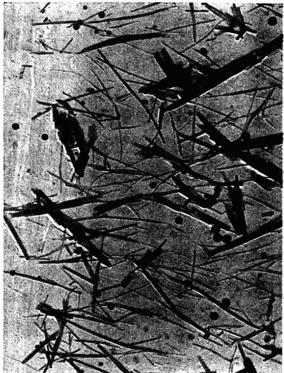
Figure 20. Electron Micrograph of Silica Replica-Dye Crystal Specimen from Steamed Pink Dyeing, 7500 \times
