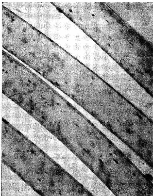
Figure 2. Photomicrograph of Steamed Yellow Dyeing, 750 \times
