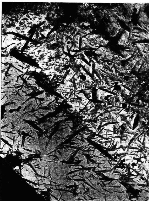
Figure 11. Electron Micrograph of Silica Replica-Dye Crystal Specimen from Original Brown Dyeing, 7500 \times
