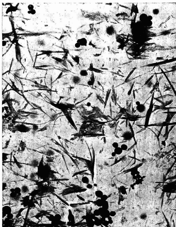
Figure 7. Electron Micrograph of Silica Replica-Dye Crystal Specimen from Original Yellow Dyeing, 7500 \times
