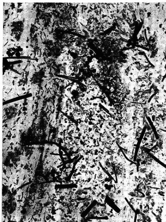
Figure 12. Electron Micrograph of Silica Replica-Dye Crystal Specimen from Original Brown Dyeing, 7500 \times
