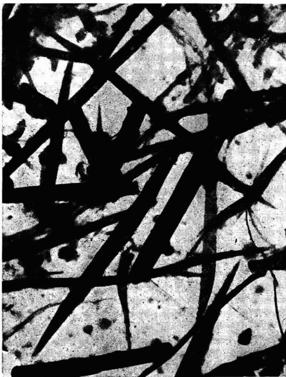
Figure 9. Electron Micrograph of Silica Replica-Dye Crystal Specimen from Steamed Yellow Dyeing, 7500 \times
