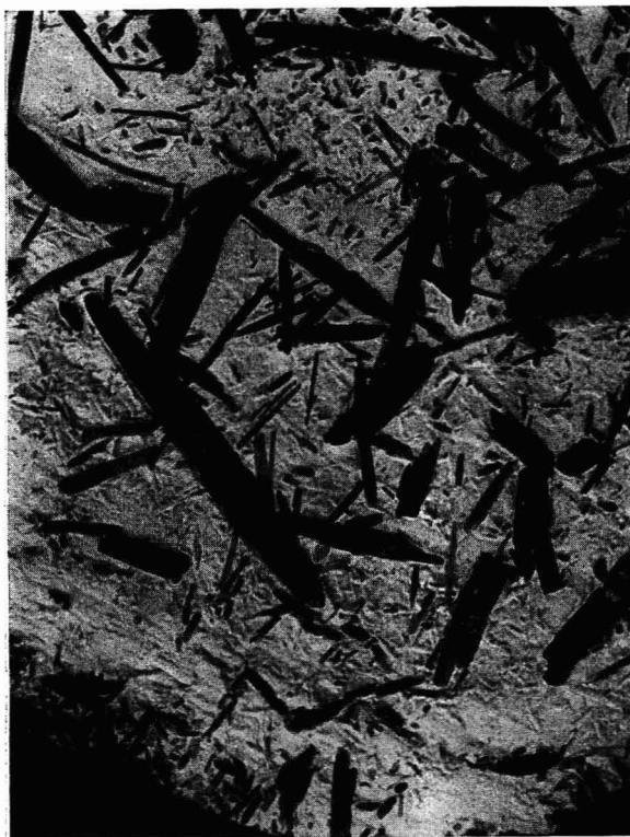
Figure 15. Electron Micrograph of Silica Replica-Dye Crystal Specimen from Steamed Brown Dyeing, 7500 \times
