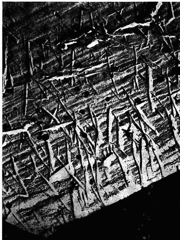
Figure 6. Electron Micrograph of Silica Replica of Steamed Pink Dyeing
